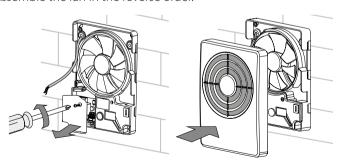
6. Fix the fan with the screws.
