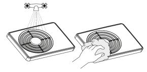
2. Remove the front panel. Clean the fan blades with a soft dry cloth or brush.
