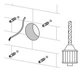
7. Remove the cover to access the terminal block and connect the fan to power mains according to the wiring diagram. Assemble the fan in the reverse order
